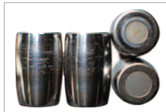
Fig. 35 Scoring on the Roller End Face
