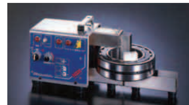
Fig. 5 Heating by bearing heater
