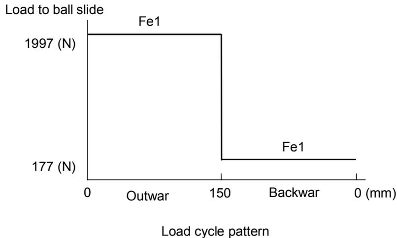
You can have the mean effective load by an equation below as the load pattern fits “(1) When the load and running distance vary stepwise” in Page A162 of the catalog.
