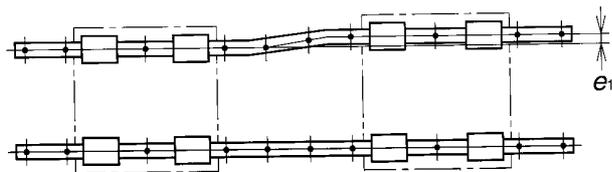
Inclination of two rails:  $e_1$
