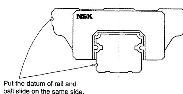
\*Interchangeable linear guides : Thanks to precise control of positions of the ball grooves on a rail and on a ball slide, these components can be randomly matched (interchangeability).
