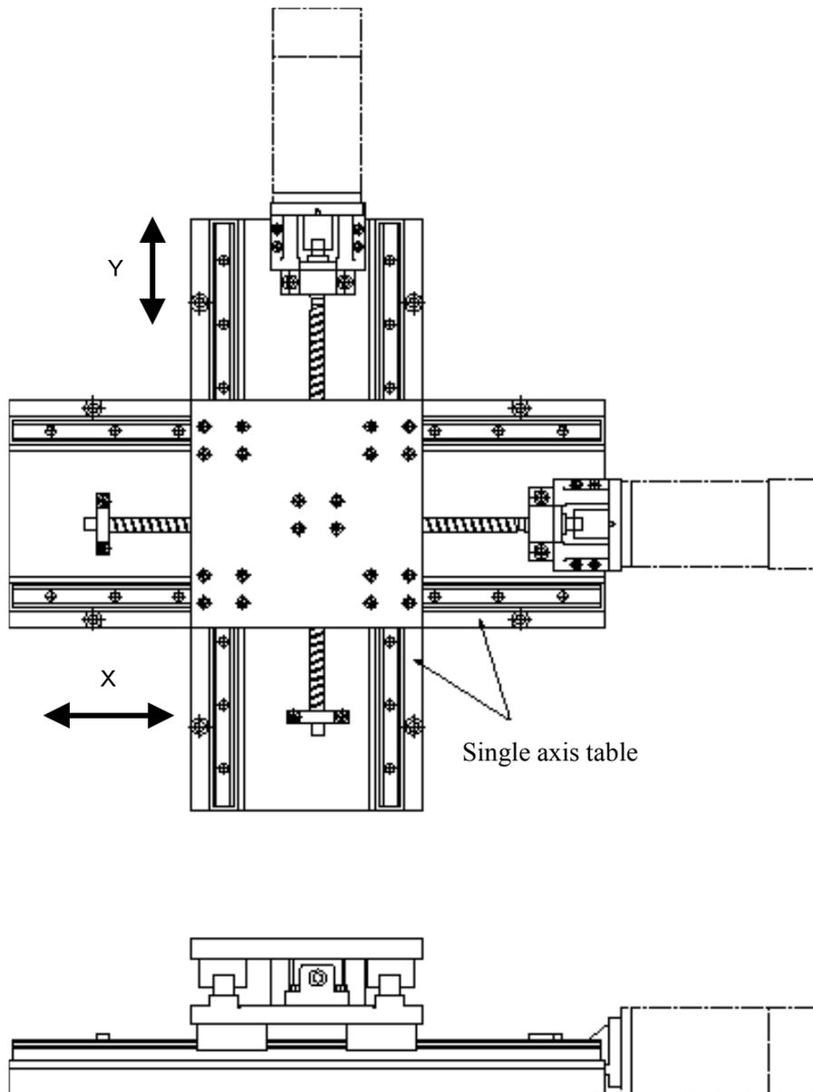
The linear guides are used as a guide to move a machine table in the direction of its X or Y axis accurately. Semiconductor manufacturing equipment or inspection apparatus that requires high precision in its positioning is one of their good application examples.
