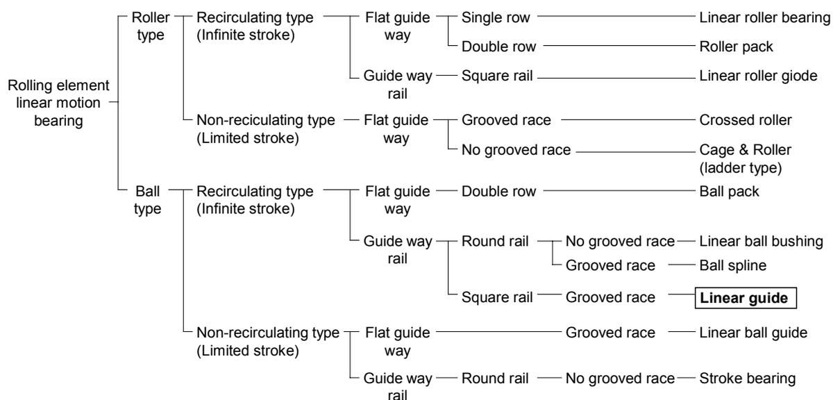
The above family tree indicates that the linear guides are positioned as "a unit component capable to guide a ball slide to make its stroke infinite by recirculating balls."
