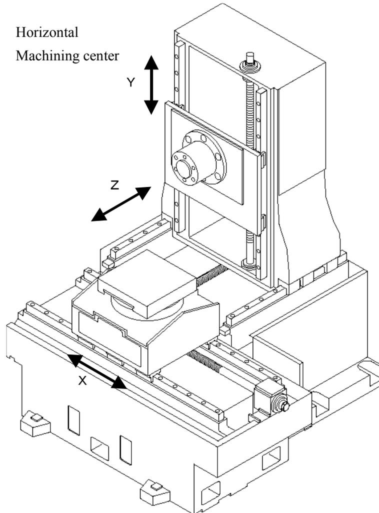
Linear guides are used to guide each table in the X, Y or Z direction in this application. For example, in the case of a machine tool for cutting, linear guides are selected to cope with temperature rise and durability issues associated with the needs to make feed speed (rapid traverse, cutting feed) ever faster, that cannot be accomplished by the sliding contact linear motion bearing. Besides, the use of linear guides will offer easiness in maintaining accuracy for a long time.
