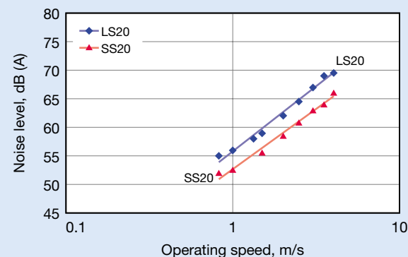
Fig. 2 Noise level comparison between LS20 and SS20
