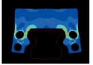
Example of bearing deformation analysis
